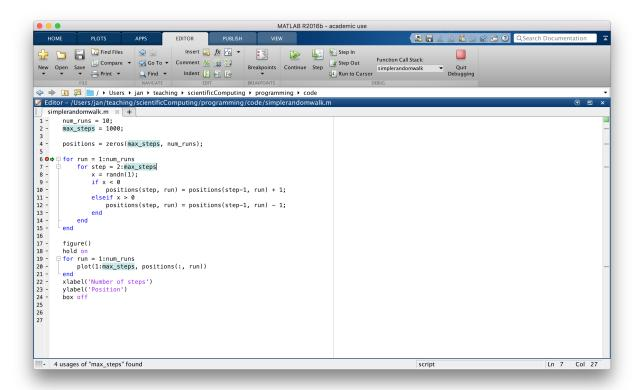
**Figure 2.1:** Screenshot of the MATLAB<sup>©</sup> m-file editor. Once a file is saved and passes the syntax check (the indicator in the top-right corner of the editor window turns green or orange), a breakpoint can be set. Breakpoints can be set either using the dropdown menu on top or by clicking the line number on the left margin. An active breakpoint is indicated by a red dot. The line at which the program execution was stopped is indicated by the green arrow.
