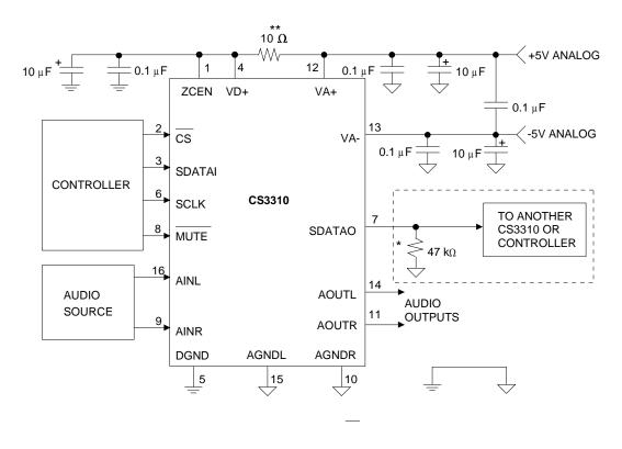
\*Required to terminate  $\underline{SDATAI}$  due to high impedance state of SDATAO when  $\overline{CS}$  is high.
