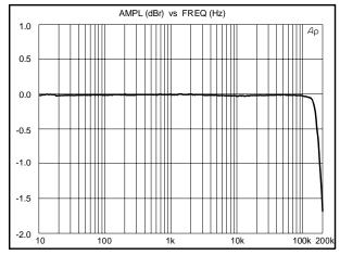
Figure 8. Frequency Response Full Scale Input
