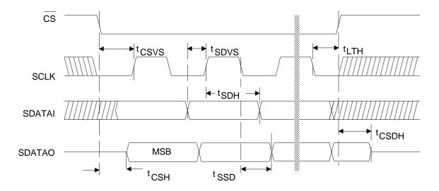
Figure 1. Serial Port Timing Diagram
