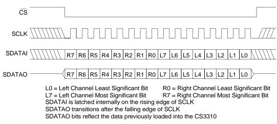
Figure 3. Serial Port Timing
