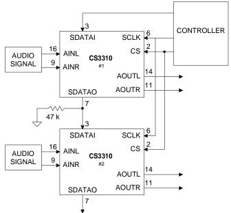
Figure 4. Daisy Chaining Diagram
