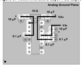
Figure 5. Recommended 2-Layer PCB Layout
