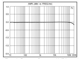
Figure 9. Frequency Response -20 dB Input
