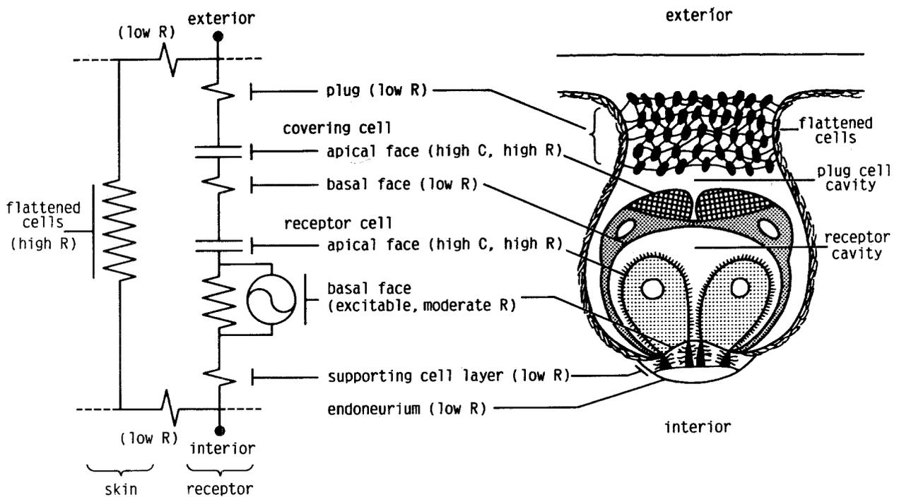
Fig. 13. Diagram of the receptor and its probable electrical equivalent circuit.
